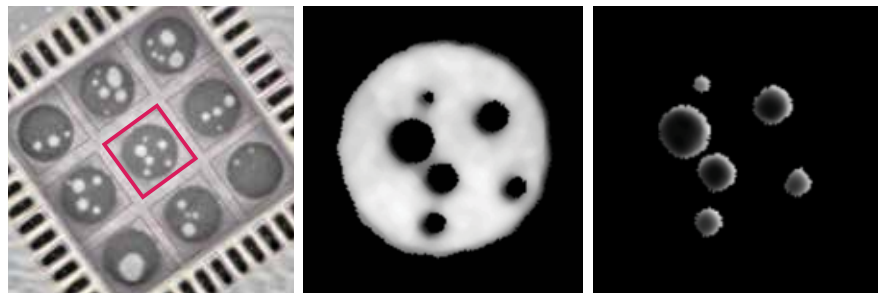
Solder voiding inspection and analysis using 3D and CT images
