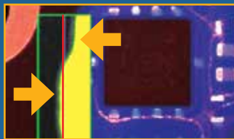
Spill & Insufficient Coating
