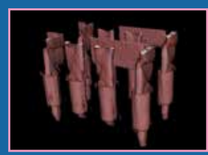
Press-fit 3D CT Inspection
