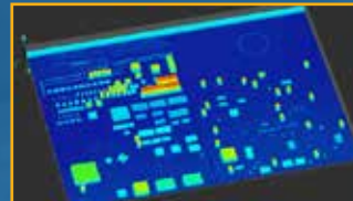
Whole Board 3D Data Flatness measurement
