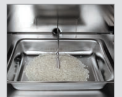
Specimen temperature display with PT 100 sensor (KBF | KBF P | KBF LQC | KMF)
