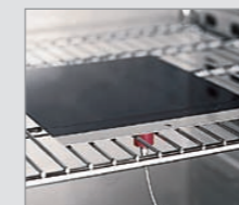
Temperature measurement of the specimen (ED | FD | FED | FP | M | FDL | MDL | VD | VDL)
