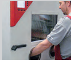
BINDER INDIVIDUAL MK with openings in the door for manual access, which is convenient when working with test specimens without disturbing the climatic conditions
