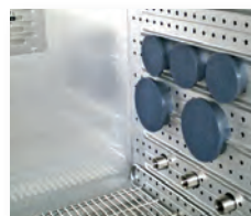
Climatic simulation chamber with various access ports for multiple instrument connection leads
