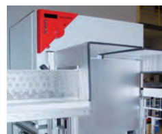
Integrated drying oven in a conveyor operation
