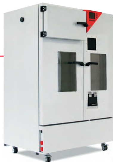
Climatic simulation chamber with additional windows, doors and access ports to accommodate the various instrument connection leads
