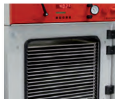
Vacuum drying oven with specific shelves for the placement of large numbers of very flat specimens
