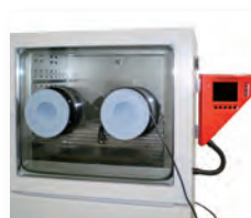
Climatic simulation chamber with full-view glass door and manual access openings
