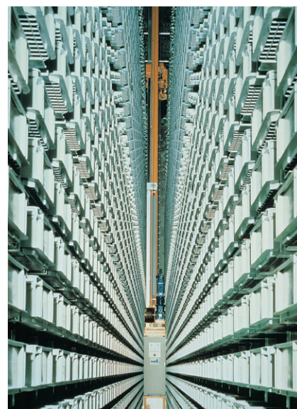
Typical use for heavy-duty-base containers in a high bay warehouse, where minimal base deflection is essential.
